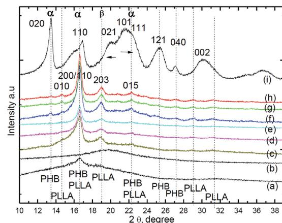
**Figure 9.** WAXS diffraction curves of PLLA, PPC and different compositions PLLA/PPC/PHB/PVAc/Plasticizer) blends, (a) (100/0/0/0/0); (b) (0/100/0/0/0) (c) (80/20/0/0/0); (d) (75/25/0/0/0); (e) (70/30/0/0/0); (f) (45/20/15/10/10); (g) (35/25/15/10/15); (h) (25/30/15/10/20); (i) (0/0/100/0/0) w/w).
