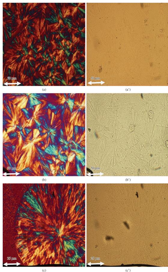
**Figure 5.** Spherulitic morphology of (PLLA/PPC/PHB/PVAc/TBC) blends, at 120 °C crystallization temperatures: with optical polarizer (a) blend 6, (b) blend 7, (c) blend 8; without optical polarizer (a') blend 6, (b') blend 7 (c') blend 8.
