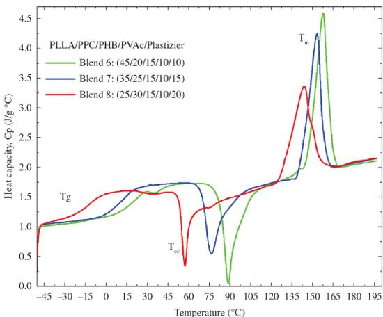
**Figure 3.** DSC; second heating of (PLLA/PPC/PHB/PVAc/TBC) blends with different compositions.
