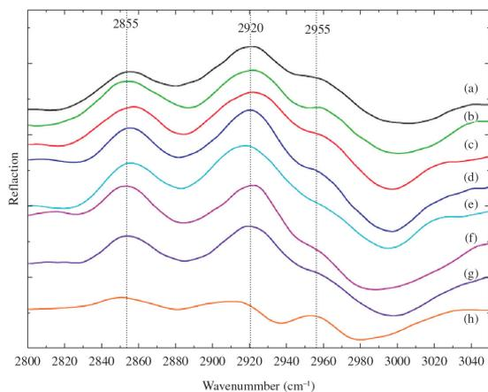
**Figure 8.** FT-IR; spectra of PLLA, PPC and different compositions PLLA/PPC/PHB/ PVAc/ Plasticizer) blends from  $2800$  to  $3050\text{ cm}^{-1}$ , (a) (100/0/0/0/0); (b) (80/20/0/0/0); (c) (75/25/0/0/0); (d) (70/30/0/0/0); (e) (45/20/15/10/10); (f) (35/25/15/10/15); (g) (25/30/15/10/20); (h) (0/100/0/0/0) w/w).
