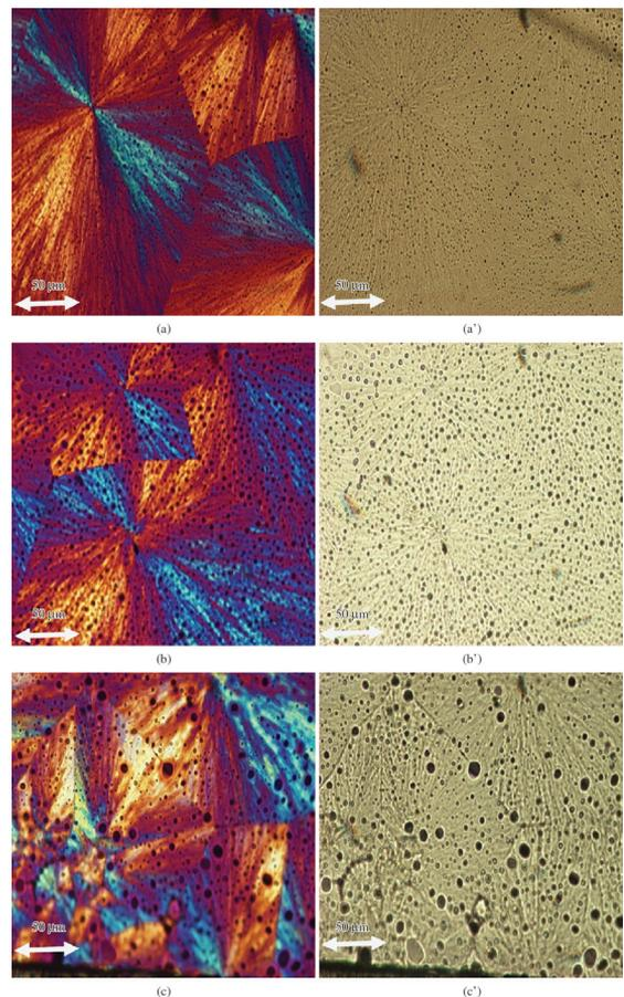
**Figure 4.** Spherulitic morphology of (PLLA/PPC) blends, at  $120\text{ }^\circ\text{C}$  crystallization temperatures: with optical polarizer (a) blend 1, (b) blend 2, (c) blend 3; without optical polarizer (a') blend 1, (b') blend 2 (c') blend 3.
