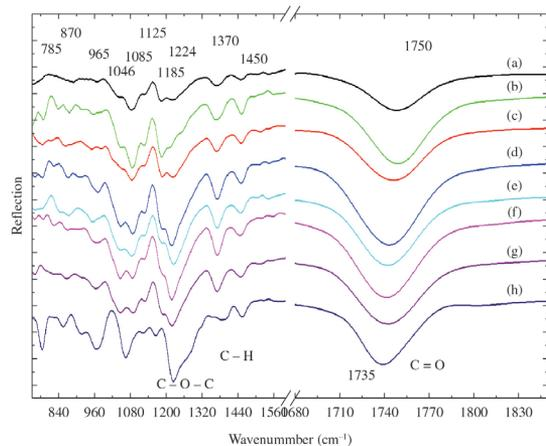
**Figure 7.** FT-IR spectra of PLLA, PPC and different compositions PLLA /PPC /PHB/ PVAc/ Plasticizer) blends from 900 to  $1850\text{ cm}^{-1}$ , (a) (100/0/0/0/0); (b) (80/20/0/0/0); (c) (75/25/0/0/0); (d) (70/30/0/0/0); (e) (45/20/15/10/10); (f) (35/25/15/10/15); (g) (25/30/15/10/20); (h) (0/100/0/0/0) w/w).
