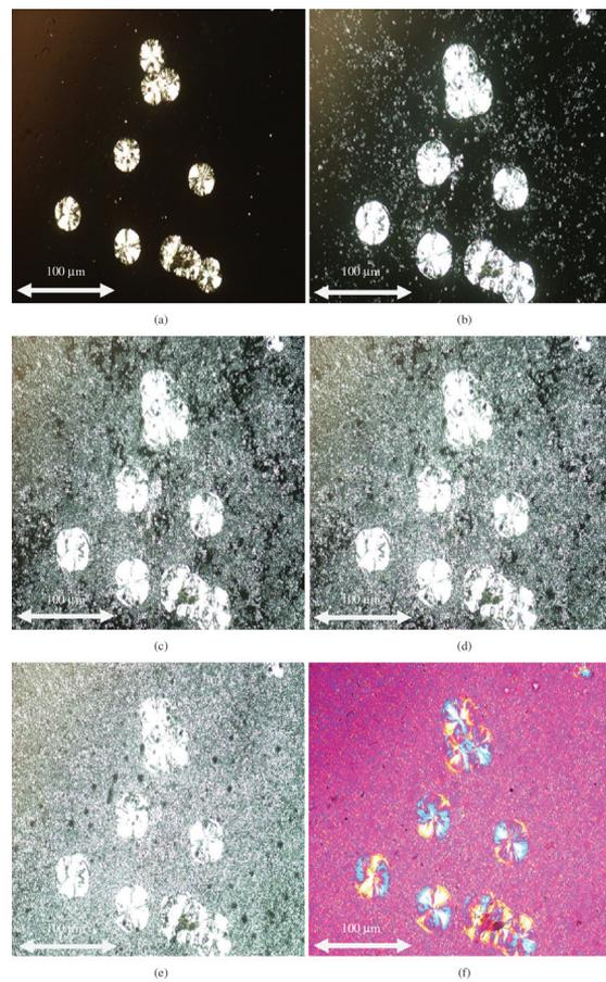
**Figure 6.** Polarized optical microscopy of spherulite texture of blend 7, crystallized isothermal at 120 and then cooled at 80 °C after different time (a) 2, (b) 3 min, (c) 5 min, (d) 6 min, (e) 7 min, (f) 8 min with 1/4  $\lambda$  and tint plate.
