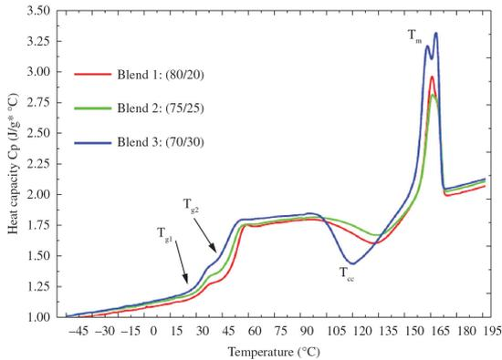
**Figure 1.** DSC; second heating of (PLLA/PPC) blends with different compositions.
