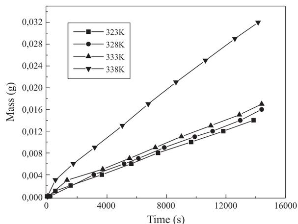
Figure 6. Permeability plot for ethanol at different temperatures.
