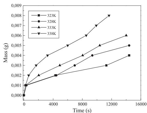
Figure 7. Permeability plot for n-propanol at different temperatures.
