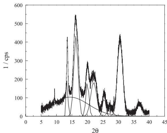
Figure 1. X-Ray Diffractogram for PHB.
