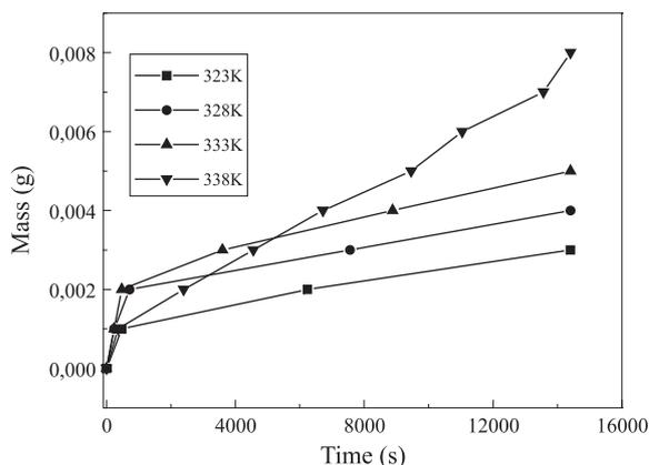
Figure 4. Permeability plot for water at different temperatures.
