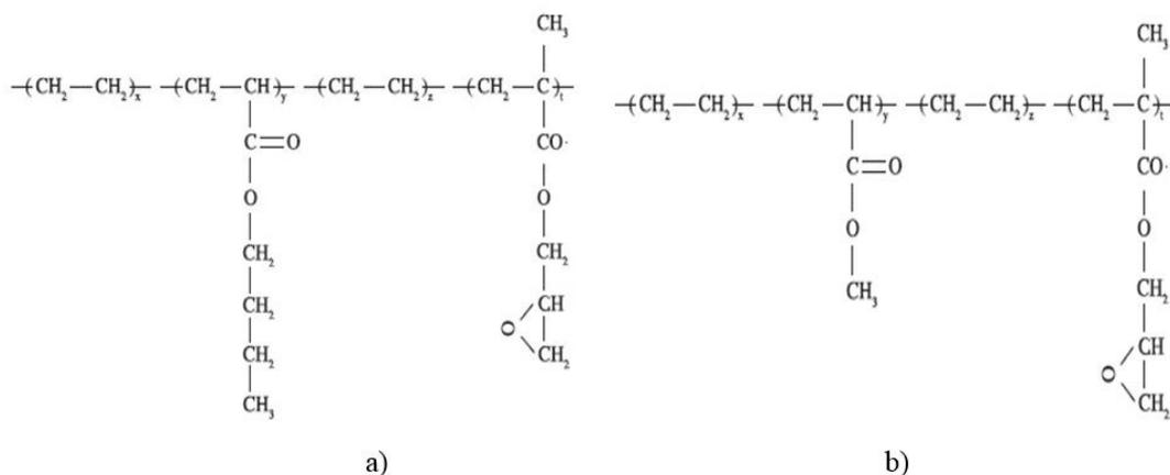
Figure 2. Molecular structure of (a) ethylene-butyl acrylate-glycidyl methacrylate terpolymer and (b) ethylene-methyl acrylate-glycidyl methacrylate terpolymer (adapted from Brito et al.<sup>[11]</sup>).
