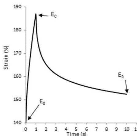
Figure 3. Deformations E<sub>0</sub>, E<sub>C</sub> and E<sub>R</sub> for one creep and recovery cycle of the MSCR test.
