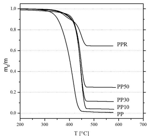
Figure 3. TGA curves of the composites and of the PP.
