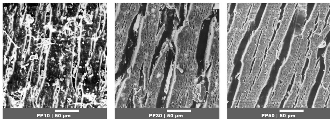
Figure 8. Micrograph of the composites surface after 120 days environmental exposure.
