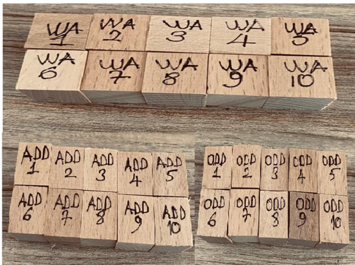
Figure 1. Image of control specimens (WA: Water absorption; ADD: Air-dry density; ODD: Oven-dry density).
