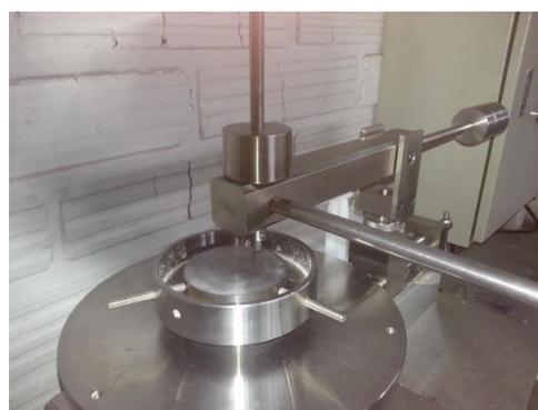
Figure 2. Pin on disc machine.
