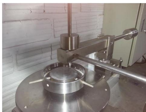
Figure 2. Pin on disc machine.
