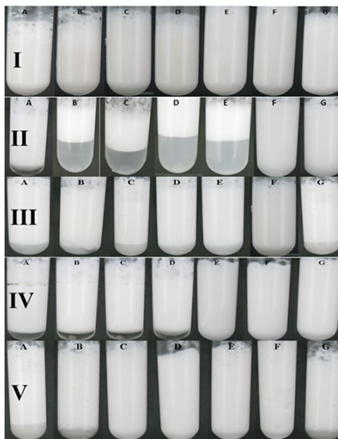
Figure 2. Visual appearances of o/w emulsions containing 10% v/v coconut oil and solutions at the seventh days of quiescent storage after their formation, when: (I) 3% w/v Lf; (II) 3% w/v OVA; (III) 2.25-0.75% w/v OVA:Lf; (IV) 2.25-0.75% w/v Lf:OVA; (V) 1.5-1.5% w/v Lf:OVA, when (A) pH 2.0; (B) 3.0; (C) pH 4.0; (D) pH 5.0; (E) pH 6.0; (F) pH 7.0; and (G) pH 8.0.
