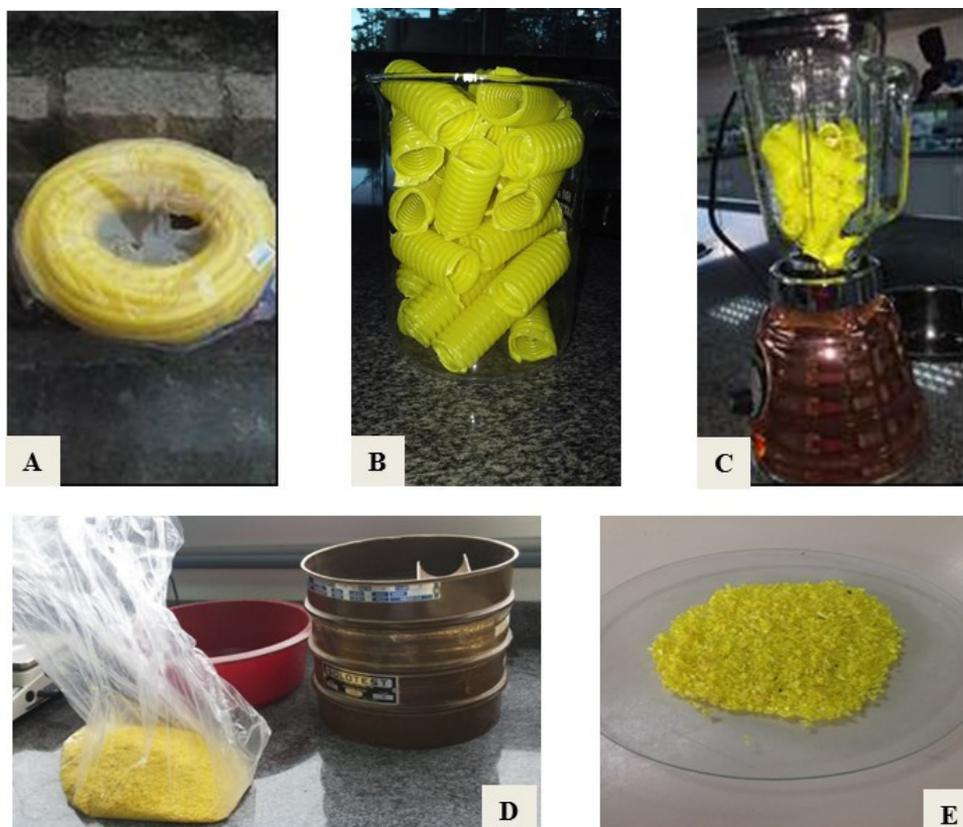
**Figure 1.** (A) Flexible PVC conduit; (B) pieces of conduit cuts; (C) pieces for grinding; (D) tritured conduit and sieves for particle size classification; (E) conduit powder with particle size less than 1.18 mm.
