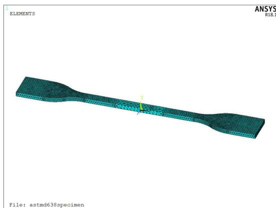
**Figure 6.** Meshing of tensile specimen in ANSYS.
