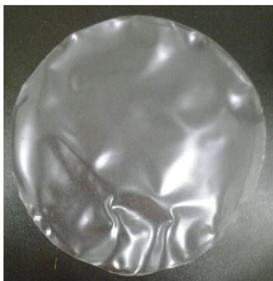
**Figure 4.** Nanobiocomposites obtained by the incorporation of 0.5% coconut cellulose nanocrystals in a manioc starch matrix plasticized with glycerol (FM05).
