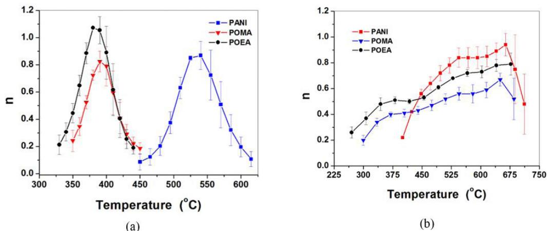
Figure 6. Flinn-Wall-Ozawa exponent ( $n$ ) versus temperature for PANI (Polyaniline) and its derivatives POEA (Poly(o-ethoxyaniline)) and POMA (Poly(o-methoxyaniline)) under (a) nitrogen and (b) oxygen atmosphere.
