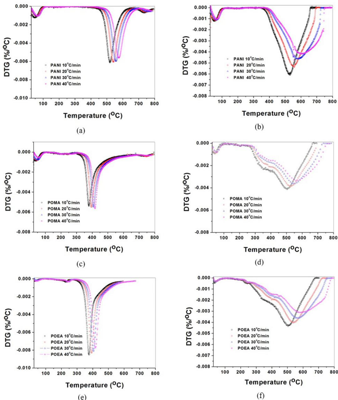
**Figure 4.** First derivative thermogravimetric (DTG) curves as a function of the heating rates for PANI (Polyaniline) and its derivatives POEA (Poly(o-ethoxyaniline)) and POMA (Poly(o-methoxyaniline)) under nitrogen (a, c, e) and oxidative (b, d, f) atmosphere.
