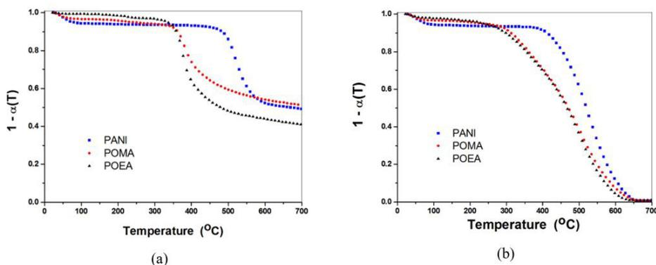
**Figure 1.** Thermogravimetric curves showing the stepwise degradation of conducting PANI (Polyaniline) and its derivatives POEA (Poly(o-ethoxyaniline)) and POMA (Poly(o-methoxyaniline)) under: (a) nitrogen and (b) oxidative atmosphere at a heating rate of 10°C/min.
