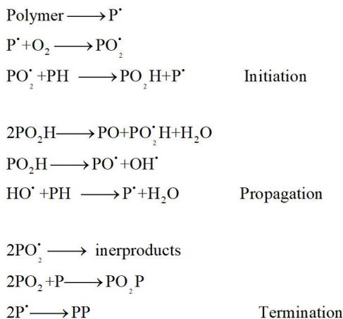
Figure 5. Scheme of general degradation of polymers by oxidation<sup>[27]</sup>.
