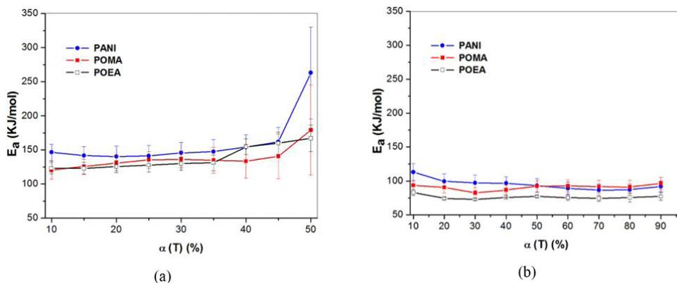
**Figure 3.** Curve vs.  $E_a$ .  $\alpha(T)$  of conducting PANI (Polyaniline) and its derivatives POEA (Poly(o-ethoxyaniline)) and POMA (Poly(o-methoxyaniline)) in the atmosphere (a) nitrogen and (b) oxygen.
