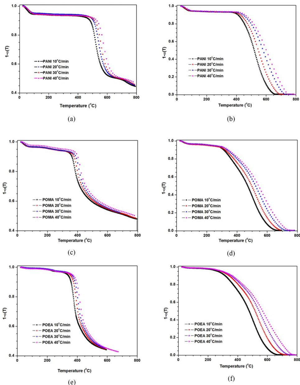
**Figure 2.** Thermogravimetric curves of PANI (Polyaniline) and its derivatives POEA (Poly(o-ethoxyaniline)) and POMA (Poly(o-methoxyaniline)) under nitrogen atmosphere (a, c, e) and oxidative (b, d, f) atmosphere at the decomposition rates of 10, 20 30 and 40 ° C/min.
