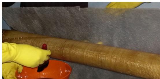
Figure 2. Wrapping of surface mat.
