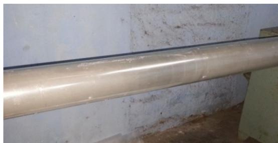
Figure 1. Terphane releasing film wounded mandrel.
