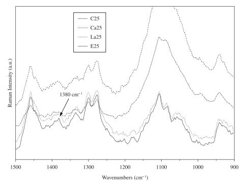
Figure 3. Raman spectra of samples containing 25% glycerol in TPS (partial of 1000 to 1500 cm<sup>-1</sup>).
