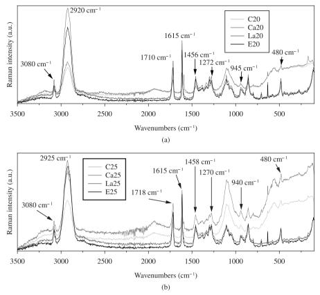
Figure 2. Raman spectra of the samples containing 20% glycerol in TPS (a) and 25% glycerol in TPS (b).
