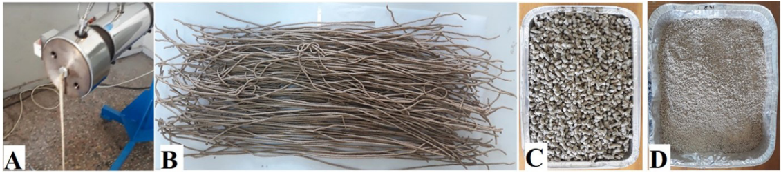
Figure 2. Extruder die (A), extruded blend (B), pellets (C), and ground blend (D).
