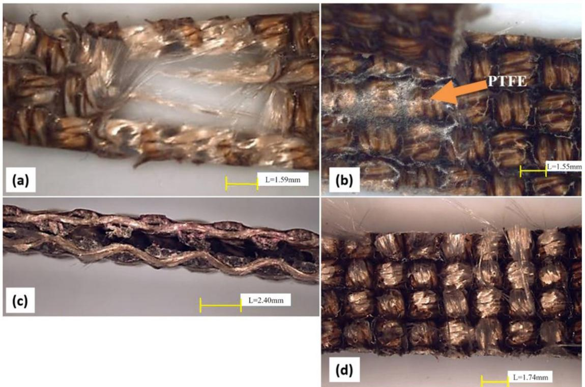
**Figure 5.** Fracture surface of the samples submitted to tensile test for (a) polymeric composite blankets without welding, (b) top view of the specimen welded at 398.8 °C (750 °F) for 4 minutes with no load applied, (c) side view of the specimen welded at 371 °C (700 °F) for 4 minutes with a load of 11.5 kgf and (d) observation of the exposed fibers of the specimen welded at 398.8 °C (750 °F) for 2 minutes with a load of 11.5 kgf.
