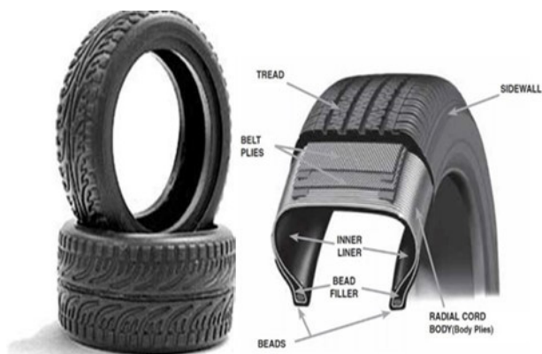
Figure 1. Typical passenger car tire and components of a run flat tire [6].
